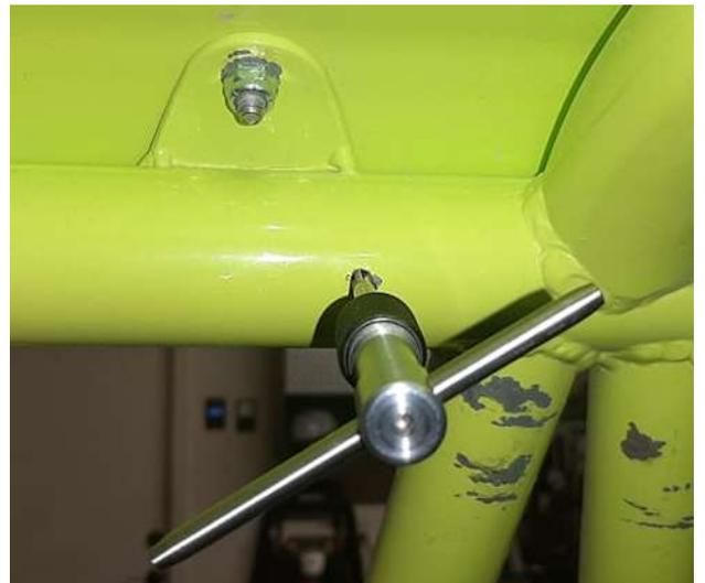
If installing a Rivet Nut is new to you, here is a great info page and a video to watch. It includes how to make the tool for just a couple of bucks too. Just use the correct size fasteners based on your choice of Metric or Imperial.
