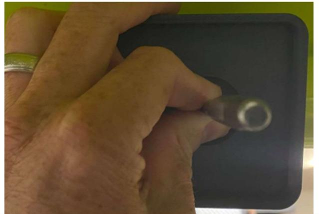
Drill a hole to accept the proper sized fastener or Rivet Nut. It is always suggested you drill a practice whole and tap it in another material prior to drilling into your cage. Ensure you drill the hole in the same plane as your screw will need to enter the tube. It should be square to the face of the mount when you had it at the viewing angle you desire.
