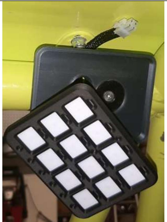
**Loosely install the bolt making sure the Switch-Pro wire harness is in the channel on the back of our mount.**
